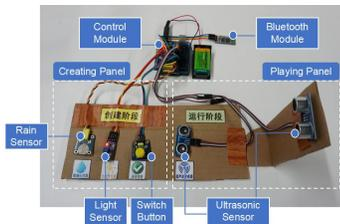
Figure 6: Control Panel consists of control module, Bluetooth module and two subpanels.
